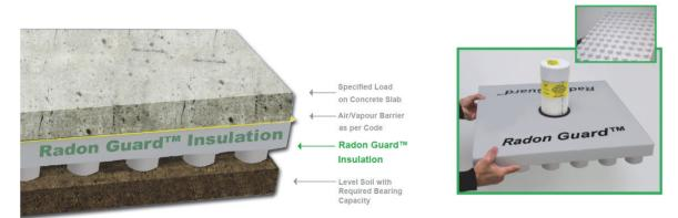
Radon Guard® insulation is a patented sub-slab depressurization panel with a pattern of circular legs on the underside that allows for soil gas removal, insulation and a capillary break between the ground and the air barrier system.<sup>2</sup> This bulletin provides guidance on recommended *PlastiSpan*<sup>®</sup> insulation types based upon total specified loads calculated using Limit States Design as per National Building Code of Canada (NBCC) 2010 and 2015.
